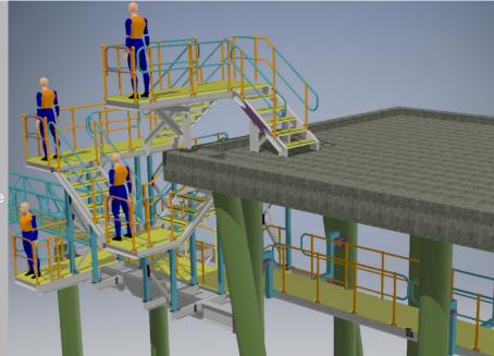
Following initial feasibility studies, PEA also completed detailed design of the vessel unloading sand conveyor and dolphin access walkways. In addition, PEA designed a new vessel access system which allows for safe access on and off the vessels by considering the height of the tides and the changing freeboard during unloading.
