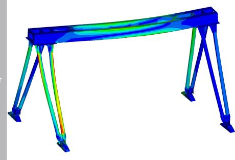
Practical Engineering undertook the design and analysis of the main structural members in addition to detail design of the 65t crane.
