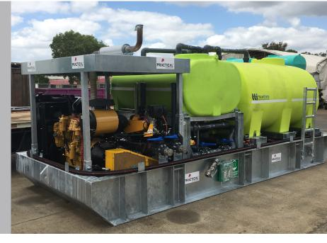
The skid-mounted unit enables gas well operators to flush wells without having to rely on the availability of rigs or cranes. This unit can be permanently mounted on a truck and allow well operators to perform flush by operations in record time minimising OPEX costs, improving efficiency and reducing safety risks associated with rigs and cranes. It consists of a self-powered pump and tank arrangement that stores the required water and chemical on board.
